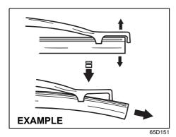
NOTE: Do not flex the wiper blade frame end more than necessary. If you do, it can break off.
