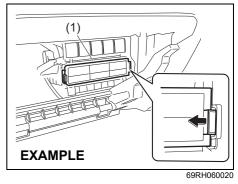
3) Slide the tab of the holder (1) in an arrow direction and remove the holder.
