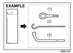
1) Pick up the towing hook (1), jack handle (2) and wheel brace (3) that are stowed in luggage compartment.
