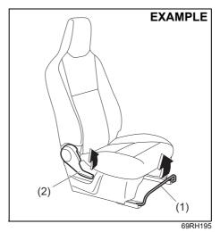
**Seat position adjustment lever (1)**Pull the lever up and slide the seat.
