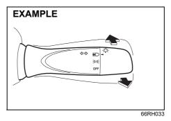
With the headlights on, push the lever forward to switch to the high beams (main beams) or pull the lever toward you to switch to the low beams. When the high beams (main beams) are on, a light on the instrument cluster will come on, to momentarily activate the high beams (main beams) as a passing signal, pull the lever slightly toward you and release it when you have completed the signal.
