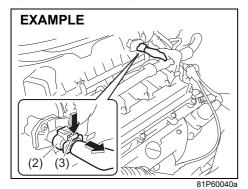
2) To disconnect the coupler (2), pull the release lever (3) toward you and then push the lever down.
