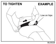
To tighten the belt, pull the free end of the belt across alongside the lap strap.
