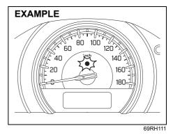
This light will blink with the ignition switch in "LOCK" or "ACC" position. The blinking light is intended to deter theft by leading others to believe that the vehicle is equipped with a security system.
