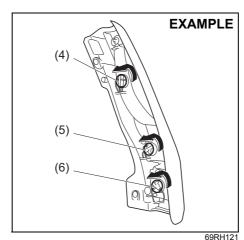
2) To remove the bulb holder of the tail/ brake light (4), the turn signal light (5) or the reversing light (6) from the light housing, turn the holder counterclockwise and pull it out.
