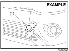
The towing hook (1) is provided on the front of the vehicle for use in emergency situations only.
