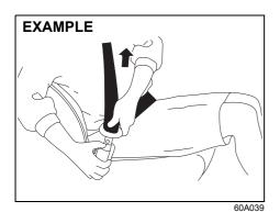
To unfasten the seat belt, push the red "PRESS" button on the buckle and retract the belt slowly while holding the belt or/and the latch plate.
