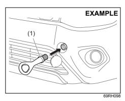
3) Install the towing hook (1) by hand.
