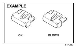
Always replace a blown fuse with a fuse of the correct amperage. Never use a substitute such as aluminum foil or wire to replace a blown fuse. If you replace a fuse and the new one blows in a short period of time, you may have a major electrical problem. Have your vehicle inspected immediately by a Maruti Suzuki authorised workshop.
