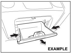
1) To approach the air conditioner filter, remove the glove box by pressing both sides of the glove box inward and pulling it out.
