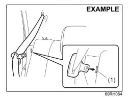
1) Insert the latch plate of the outboard lap-shoulder belts into the slit (1).
