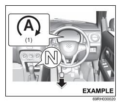
After the vehicle has stopped with the clutch pedal depressed and the gearshift lever shifted to "N", and then release the clutch pedal, the engine will stop automatically.
