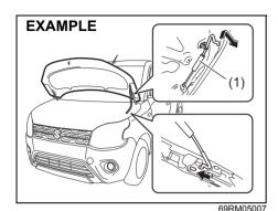
While holding the hood, pull the prop rod out from the holding clip, and then insert the end of the rod into the designated hole.
