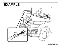
3) While holding the hood, pull the prop rod out from the holding clip, then insert the end of the rod into the designated hole in the hood.
