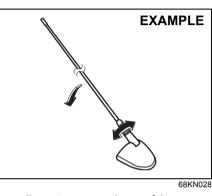
The radio antenna on the roof is removable. To remove the antenna, turn it counterclockwise. To reinstall the antenna, turn it clockwise firmly by hand.
