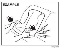
4) Grasp the front of the child restraint and push the child restraint forcefully to latch the connecting bars. Check that they are securely latched by trying to
