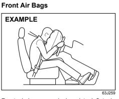
Front air bags are designed to inflate in severe frontal collisions when the ignition switch is in the "ON" position or the ignition mode is "ON".
