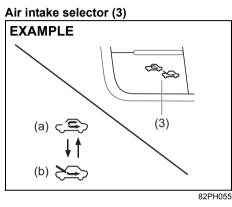
Push the air intake selector (3) to change between the following modes.
