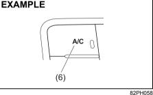
The air conditioning switch (6) is used to turn on and off the air conditioning system only when the blower is on. To turn on the air conditioning system, push in the switch; "A/C" will appear on the display and the indicator on the switch will come on. To turn off the air conditioning system, push in the switch again; "A/C" and the indicator will go off.
