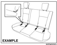
Your vehicle is equipped with the lower anchorages in the rear seat outboard seating positions for securing a ISOFIX type of child restraints with the connecting bars. The lower anchorages are located where the rear of the seat cushion meets the bottom of the seatback.
