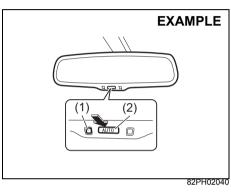
You can adjust the auto dimming rearview mirror by hand so you can see to the rear of your vehicle in the mirror. This rearview mirror has a function of automatically reducing glare from the lights of vehicles behind you. The function works when the ignition mode has been changed to "ON" by pressing the engine switch.
