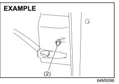
2) To remove and install the bulb of the glove box light (2), simply pull out or push in the bulb.
