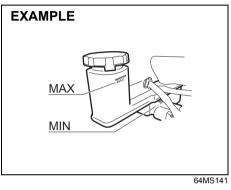
Check the clutch pedal for smooth operation and clutch fluid level from time to time. If clutch dragging is felt with the pedal fully depressed, have the clutch inspected by a Maruti Suzuki authorised workshop. If the clutch fluid level is near the "MIN" line, fill it up to the "MAX" line with Maruti Genuine Brake Fluid (MGBF) or DOT 3.
