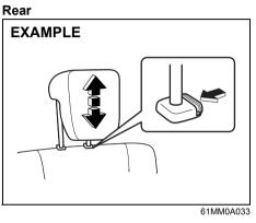
To raise the rear head restraint, pull upward on the restraint until it clicks. To lower the restraint, push down on the restraint while holding in the lock lever. If a head restraint must be removed (for cleaning, replacement, etc.), push in the lock lever and pull the head restraint all the way out.
