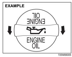
Remove the oil filler cap and pour oil slowly through the filler hole to bring the oil level to the upper limit on the dipstick. Be careful not to overfill. Too much oil is almost as bad as too little oil. After refilling, start the engine and allow it to idle for about a minute. Stop the engine, wait about 5 minutes and check the oil level again. **Changing Engine Oil and Filter**
