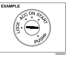
The ignition switch has the following four positions:
