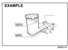
Check the brake fluid level by looking at the reservoir in the engine compartment. Check that the fluid level is between the "MAX" and "MIN" lines. If the brake fluid level is near the "MIN" line, fill it up to the "MAX" line with Maruti Genuine Brake Fluid (MGBF) or DOT 3 brake fluid. We highly recommend to use "Maruti Genuine Brake Fluid" (MGBF).
