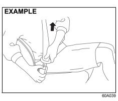
To unfasten the seat belt, push the button on the buckle and retract the belt slowly while attaching a hand to the belt or/and the latch plate.
