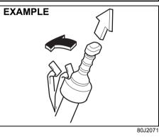
6) The handle of the A/T fluid dipstick is colored red for easy identification. Remove the dipstick, wipe the oil off with a clean cloth and push it back in until the cap seats. Then pull out the dipstick.
