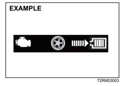
While decelerating your vehicle, the ISG generates electricity without engine power. This reduces engine loads and improves fuel consumption.
