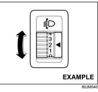
Level the headlight beam according to the load condition of your vehicle by turning this switch. The chart below shows the appropriate switch position for different vehicle-load conditions.
