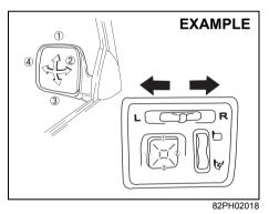
The switch to control the electric mirrors is located on the instrument panel. You can adjust the mirrors when the ignition switch is in the "ACC" or "ON" position, or the ignition mode is "ACC" or "ON". To adjust the mirrors:
