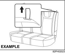
Pull up the release straps on the top of the seat(s), and fold the seatback forward.
