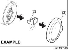
1) Open the engine hood. Remove the sealing rubber (3) and disconnect the coupler (2).
