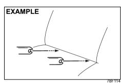
Place the child restraint in the rear seat, inserting the connecting bars to the anchorages between the seat cushion and the seatback.
