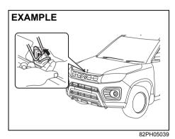
Push the under-hood release lever sideways with your finger, as shown in the illustration. While pushing the lever, lift up the engine hood.
