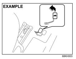
You can also unlatch the tailgate by pulling the release lever located on the outboard side of the driver's seat.
