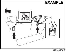
Some child restraint systems require the use of a top tether strap. Top tether anchorage brackets are provided in your vehicle at the locations shown in the illustrations.
