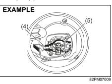
Push the retaining spring (4) forward and unhook it. Then remove the bulb (5). Install a new bulb in the reverse order of removal.
