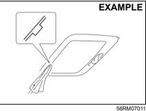
Remove the lens by using a flat blade screwdriver covered with a soft cloth as shown. To install it, simply push it back in.
