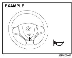
Press the horn button of the steering wheel to sound the horn. The horn will sound with the ignition switch in any position or any ignition mode.
