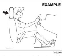
Head restraints are designed to help reduce the risk of neck injuries in the case of an accident. Adjust the head restraint to the position which places the center of the head restraint closest to the top of your ears. If this is not possible for very tall passengers, adjust the head restraint as high as possible.
