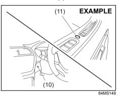
Be careful not to cover the interior temperature sensor (10) located between the steering wheel and the climate control panel, or the solar sensor (11) located at the top of the central part of the dashboard. These sensors are used by the automatic system to regulate temperature.
