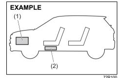
(1) Battery (lead-acid battery)(2) Lithium-ion battery
