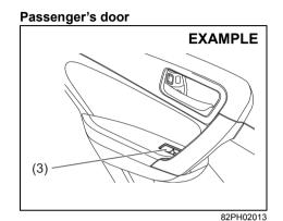
The passenger's door has a switch (3) to operate that passenger's window.
