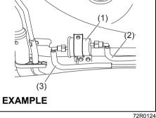
(1) Fuel filter (2) Fuel inlet hose (3) Fuel outlet hose
