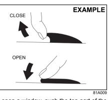
To open a window, push the top part of the switch and to close the window, lift up the top part of the switch.
