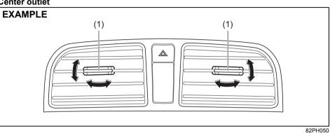
Move the knob (1) vertically or horizontally to adjust the direction of airflow as desired.
