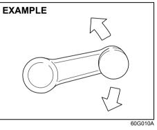
Raise or lower the door windows by turning the handle located on the door panel.
