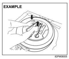
To remove the jack, hold the tire changing tool storage with one hand while pulling the jack from the centre as shown in the above illustration.
