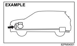
The purpose of the catalytic converter is to minimize the amount of harmful pollutants in your vehicle's exhaust. Use of leaded fuel in vehicles equipped with catalytic converters is prohibited, because lead deactivates the pollutant-reducing components of the catalyst system.
