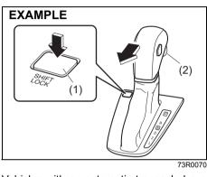
Vehicles with an automatic transaxle have an electrically operated park-lock feature. If the vehicle's battery is discharged, or there is some other electrical failure, the automatic transaxle cannot be shifted out of Park in the normal way. Jump starting may correct the condition. If not, follow the procedure described below. This procedure will permit shifting the transaxle out of Park.
