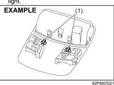
3) Rotate and remove the spot light bulb (1) from the socket. Install a new bulb in the reverse order of removal.
