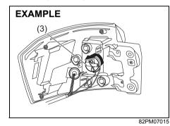
To remove the bulb holder of the turn signal light (3) from the light housing, turn the holder counterclockwise and pull it out.
