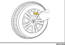
Insert a piece of cloth between the spokes of the wheel cover and try to pull the cover outward (as shown in figure). Take out the detached wheel cover from the wheel rim. For installation first match the slot at the wheel cover with the air filling nozzle of the wheel. Apply equal pressure at the circumference of the wheel cover to fix it in the wheel rim.
