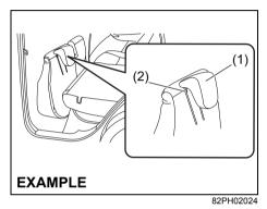
Insert the head restraint(s) (if equipped) rod (1) into the loop (2) provided on the cushion(s).
