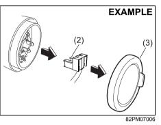
Open the engine hood.Remove the sealing rubber (3) and disconnect the coupler (2).
