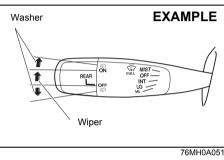
To turn the rear wiper on, twist the rear wiper switch on the end of the lever forward to the "ON" position. To turn the rear wiper off, twist the switch rearward to the "OFF" position.
