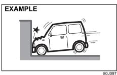
In frontal collisions with a fixed wall that does not move or deform at more than about 25 km/h Conditions when front airbags may inflate
