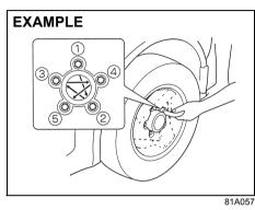
Tightening torque for wheel nut 100 Nm (10.2 kg-m, 73.8 lb-ft)
