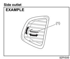
Move the knob (1) vertically or horizontally, to adjust the direction of airflow as desired.
