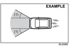
Strong impact equivalent to frontal collision such as above at left and right angles of about 30 degrees (1) or less from the front of your vehicle
