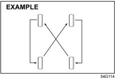
To avoid uneven wear of your tires and to prolong their life, rotate the tires as illustrated. Tires should be rotated every 10000 km. After rotation, adjust front and rear tire pressures to the specification listed on your vehicle's Tire Information Label.
