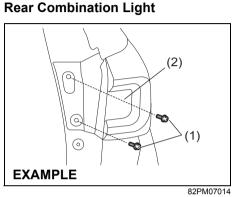
1) Remove the bolts (1) and pull the light housing (2) straight.
