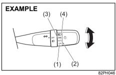
ON: Lights ON LIGHT: When it is light around the light sensor (5). DARK: When it is dark around the light sensor (5).
