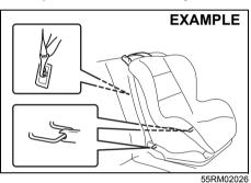
Your vehicle is equipped with the top tether anchorages. Use the top tether strap of the child restraint according to the instructions provided by the child restraint system manufacturer. Here is a general instruction:
