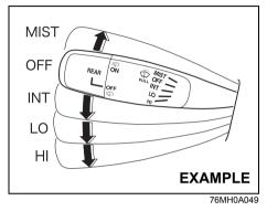
To turn the windshield wipers on, move the lever down to one of the three operating positions. In the "INT" position, the wipers operate intermittently. The "INT" position is very convenient for driving in mist or light rain. In the "LO" position, the wipers operate at a steady low speed. In the "HI" position, the wipers operate at a steady high speed. To turn off the wipers, move the lever back to the "OFF" position.
