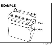
For maintenance-free battery (cap-less type), you need not add water. For traditional type battery, which has water filler caps, the level of the battery fluid must be kept between the "MAX" and the "MIN" level lines at all times. You should periodically check the battery, battery terminals, and battery hold-down bracket for corrosion. Remove corrosion using a stiff brush and ammonia mixed with water, or baking soda mixed with water. After removing corrosion, rinse with clean water.
