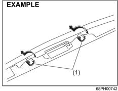
1) Turn the lens (1) counterclockwise to remove it.
