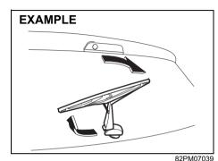
Remove the wiper frame from the wiper arm after rotating the wiper frame clockwise.
