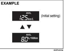
When you change the units that average fuel consumption is displayed in, the instantaneous fuel consumption units will be changed automatically.
