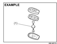
(1) Lithium disc type battery: CR2032 or equivalent
