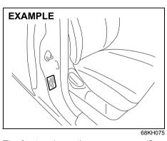
The front and rear tire pressure specifications for your vehicle are listed on the Tire Information Label. Both the front and rear tires should have the specified tire pressure.
