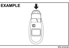
To stow the key into the remote controller, push the key in the remote controller until you hear a click.
