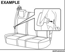
1) Insert the latch plate of the outboard lap-shoulder belts into the slit (1).
