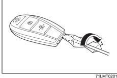
2) Insert a flat blade screwdriver covered with a soft cloth in the slot of the remote controller and pry it open.
