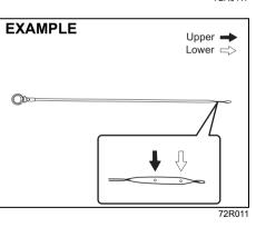
It is important to keep the engine oil at the correct level for proper lubrication of your vehicle's engine. Check the oil level with the vehicle on a level surface. The oil level indication may be inaccurate if the vehicle is on a slope. The oil level should be checked either before starting the engine or at least 5 minutes after stopping the engine.
