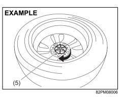
Return the spare tire back into the luggage compartment in the reverse order of removal and tighten its bolt (5) clockwise as shown in the above illustration.
