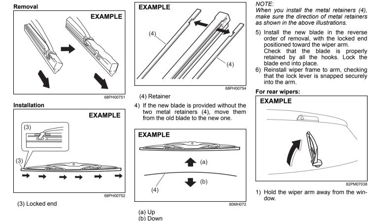
When you install the metal retainers (4), make sure the direction of metal retainers as shown in the above illustrations.
