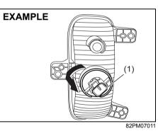
Open the engine hood and disconnect the connector. To remove the bulb holder of the front turn signal light (1) from the light housing, turn the holder counterclockwise and pull it out.
