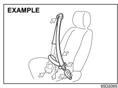
Periodically inspect the seat belts to make sure they work properly and are not damaged. Check the webbing, buckles, latch plates, retractors, anchorages, and guide loops. Replace any seat belts which do not work properly or are damaged.
