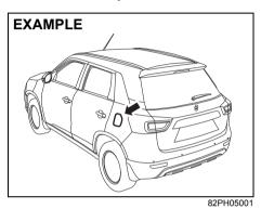
The fuel filler cap is located on the left rear side of the vehicle. The fuel filler door can be unlocked by pulling up the opener lever located on the outboard side of the driver's seat and locked by simply closing the door.
