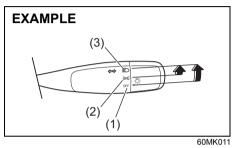
To turn the lights on or off, twist the knob on the end of the lever. There are three positions:
