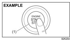
Every time you press the engine switch, the ignition mode changes as follows.
