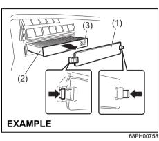
2) Remove the cover (1) and pull out the air conditioner filter (2).
