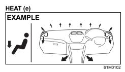
Temperature-controlled air comes out of the floor outlets, also comes out of the windshield defroster outlets and also comes slightly out of the side defroster outlets and the side outlets.
