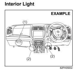
(1) Glove box light (if equipped) (2) Footwell lights (if equipped)
