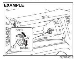
When the air conditioning system is operated with the ventilation position, you can keep items such as drinks cool in the cool box. Turn the shut dial (2) to open or close the air outlet.
