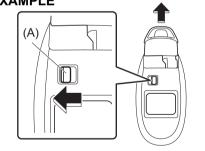
To remove the key from the remote controller, push the button (A) in the direction of
