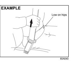
To reduce the risk of sliding under the belt during a collision, position the lap portion of the belt across your lap as low on your hips as possible and adjust it to a snug fit by pulling the shoulder portion of the belt upward through the latch plate. The length of the diagonal shoulder strap adjusts itself to allow freedom of movement.
