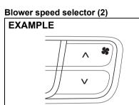
The blower speed selector (2) is used to turn on the blower and to select blower speed.
