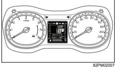
When the ignition switch is turned to the "ON" position or the engine switch is pressed to change the ignition mode to ON, the instrument panel lights come on.
