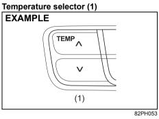
Push upper part or lower part of the temperature selector (1) to adjust the temperature. The display (9) shows the selected temperature.
