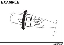
If the control lever has an "AUTO" position, you can change the system's sensitivity to rain/snow by turning the knob of the control lever forward (+) for increased sensitivity or rearward (–) for decreased sensitivity.
