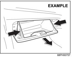
1) To approach the air conditioner filter, press inward on both sides of the glove box, pull it frontward and remove it.
