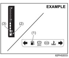
When the ignition switch is in the "ON" position or the ignition mode is "ON", this gauge gives an approximate indication of the amount of fuel in the fuel tank. "F" stands for full and "E" stands for empty.
