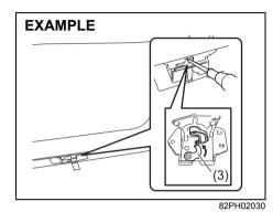
2) Push open the tailgate from inside by pushing up on the emergency lever (3) using a flat blade screwdriver or the jack handle. The tailgate will be latched again by closing the tailgate simply.
