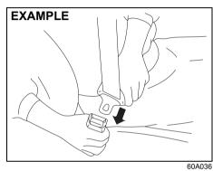
To fasten the seat belt, sit up straight and well back in the seat, pull the latch plate attached to the seat belt across your body and press it straight into the buckle until you hear a click.
