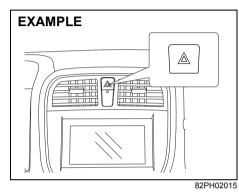
Push in the hazard warning switch to activate the hazard warning lights. All turn signal lights and both turn signal indicators will flash simultaneously. To turn off the lights, push the switch again.
