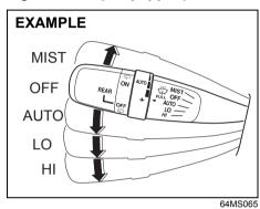
Press the engine switch to change the ignition mode to "ON". To turn the rain-sensing wipers on, move the lever down to one of the three operating positions. In the "AUTO" position (if provided), the wipers automatically operate when the wiper system senses rain or snow. In the "LO" position, the wipers operate at a steady low speed. In the "HI" position, the wipers operate at a steady high speed. To turn off the wipers, move the lever back to the "OFF" position.
