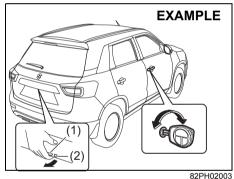
(1) Tailgate unlatch switch(2) Request switch (if equipped)
