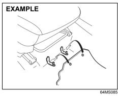
To prevent the driver's side floor mat from sliding forward and possibly interfering with the operation of the pedals, MARUTI genuine floor mats are recommended.
