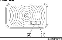
When you open the tailgate with the luggage compartment light switch in the ON position (1), the light comes on and remains on as long as you keep the tailgate open.
