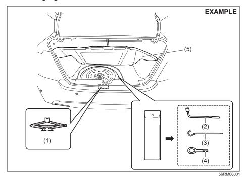
The tire changing tools are stowed in the luggage compartment, below the luggage compartment board (5). Pull the thread of the luggage compartment board upwards. The luggage compartment board can be held open by hanging the thread on the hook as shown in the above illustration. in the above illustration.
