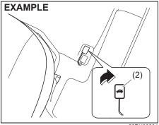
You can unlock the lid by pulling the trunk lid opener lever (2) located on the outboard side of the driver's side.
