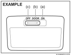
These light switches have three positions which function as described below:
