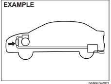
The purpose of the catalytic converter is to minimize the amount of harmful pollutants in your vehicle's exhaust. Use of leaded fuel in vehicles equipped with catalytic converters is prohibited, because lead deactivates the pollutant-reducing components of the catalyst system.
