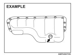
Tightening torque for drain plug 35 Nm (3.6 kg-m, 25.8 lb-ft)
