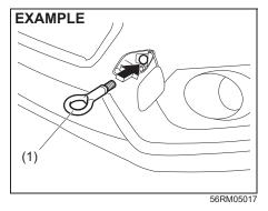
3) Screw in the towing hook (1) by hand.
