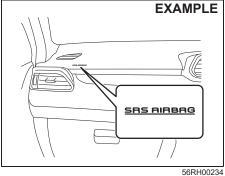
The driver's front air bag is located behind the center pad of the steering wheel and the front passenger's front air bag is located behind the passenger's side of the dashboard.
