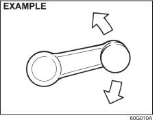
Raise or lower the door windows by turning the handle located on the door panel.
