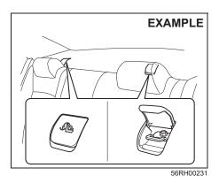
Some child restraint systems require the use of a top tether strap. Top tether anchorage brackets are provided in your vehicle at the locations shown in the illustrations.
