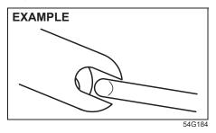
Push the child restraint toward the anchorages so that the connecting bar tips are partially hooked to the anchorages. Use your hands to confirm the position.
