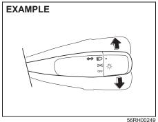
With the headlights on, push the lever forward to switch to the high beams (main beams) or pull the lever toward you to switch to the low beams. When the high beams (main beams) are on, a light on the instrument cluster will come on. To momentarily activate the high beams (main beams) as a passing signal, pull the lever slightly toward you and release it when you have completed the signal.
