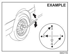
Tightening torque for wheel nut 100 Nm (10.2 kg-m, 74.0 lb-ft)
