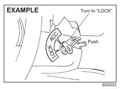
You must push in the key to turn it to "LOCK" position. It locks the ignition, and prevents normal use of the steering wheel after the key is removed.
