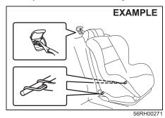
Your vehicle is equipped with the top tether anchorages. Use the top tether strap of the child restraint according to the instructions provided by the child restraint system manufacturer.
