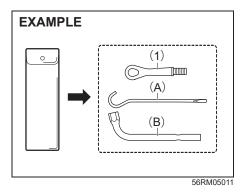
Pick up the towing hook (1), jack handle (A) and wheel wrench (B) from the luggage compartment.
