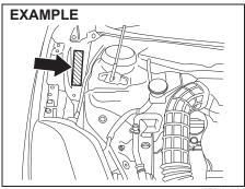
The chassis and/or engine serial numbers are used to register the vehicle. They are
