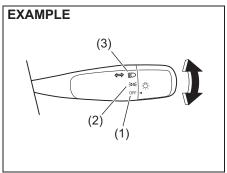
To turn the lights on or off, twist the knob on the end of the lever. There are three positions:
