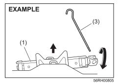
To remove the jack (1), turn its shaft counterclockwise by using jack handle (3) and pull the jack out of the storage bracket.
