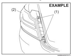
1) Remove the bolts (1) and pull the light
