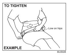
To tighten the belt, pull the free end of the belt across alongside the lap strap.
