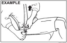
To unfasten the seat belt, push the red "PRESS" button on the buckle and retract the belt slowly while holding the belt or/and the latch plate.
