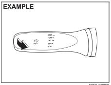
To spray windshield washer fluid, pull the lever toward you. The windshield wipers will automatically turn on at low speed if they are not already on and your vehicle is equipped with "INT" position.
