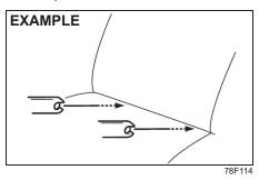
Place the child restraint in the rear seat, inserting the connecting bars to the anchorages between the seat cushion and the seatback.
