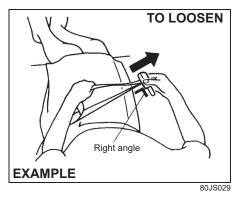
To lengthen, release the latch plate from the buckle, pull the latch plate (adjuster) in the direction of the arrow, at right angles to the belt. The latch plate should then be refitted into the buckle and the belt tightened as previously described.
