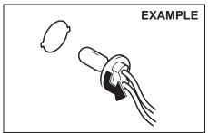
1) Open the engine hood. To remove the bulb holder of the front turn signal light or the front position light from the light housing, turn the holder counterclockwise and pull it out.
