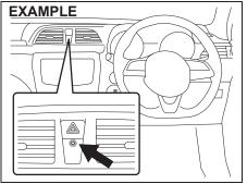
This light will blink with the ignition switch in "LOCK" or "ACC" position. The blinking light is intended to deter theft by leading others to believe that the vehicle is equipped with a security system.
