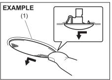
1) Remove the light housing (1) by sliding to left with your finger.
