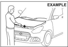
2) Lower the hood to about 20 cm above the hood latch, and then let it drop down. Check that the hood is securely latched after closing.
