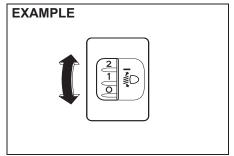
Level the headlight beam according to the load condition of your vehicle by turning this switch. The chart shows the appropriate switch position for different vehicle load conditions.
