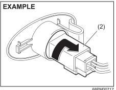
2) Turn the bulb holder (2) clockwise and pull it out from the light housing.
