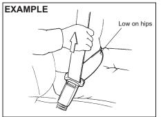
To reduce the risk of sliding under the belt during a crash, position the lap portion of the belt across your lap as low on your hips as possible and adjust it to a snug fit by pulling the shoulder portion of the belt upward through the latch plate. The length of the diagonal shoulder strap adjusts itself to allow freedom of movement.
