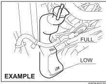
If the coolant level is below "LOW" mark. more coolant should be added. While the engine cool, remove the reservoir tank cap and add coolant until the reservoir tank level reaches "FULL" mark. Never fill the reservoir tank above "FULL" mark.
