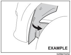
3) Open the end of the cover inside the fender.
