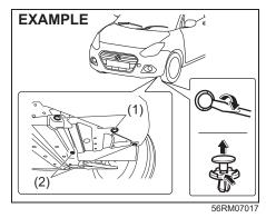
2) Remove the clips (1) and screws (2) at the bottom of bumper.
