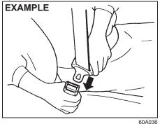
To fasten the seat belt, sit up straight and far back into the seat, pull the latch plate attached to the seat belt across your body and press it straight into the buckle until you hear a "click".
