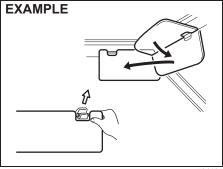
The sun visors can be pulled down to block glare coming through the windshield, or they can be unhooked and turned to the side to block glare coming through the side window.
