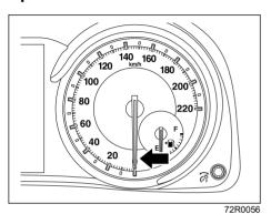
The speedometer indicates vehicle speed in km/h.
