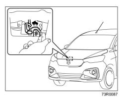
Push the under-hood release lever upward with your finger, as shown in the illustration. While pushing the lever, lift up the engine hood.
