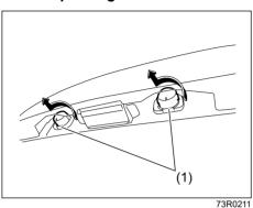
1) Remove the cover (1) by turning it counterclockwise.
