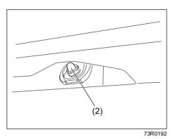
2) To remove and install the bulb of the license plate light (2), simply pull out or push in the bulb.
