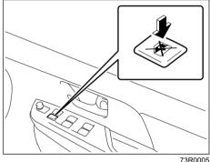
The driver's door also has a lock switch for the passenger's windows. When you push in the lock switch, the passenger's windows cannot be raised or lowered by operating any of the switches (2), (3), (4) or (5). To restore normal operation, release the lock switch by pushing again.
