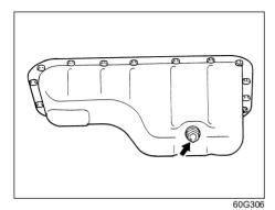
Tightening torque for drain plug 35 Nm (3.6 kg-m, 25.8 lb-ft)
