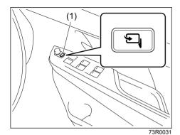
You can fold the mirrors when you park the vehicle in a narrow space. When the ignition switch is in the ACC or ON position, push the folding switch (1) to fold and unfold the mirrors.
