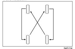
To avoid uneven wear of your tires and to prolong their life, rotate the tires as illustrated. Tires should be rotated every 10000 km. After rotation, adjust front and rear tire pressures to the specification listed in your vehicle's Tire Information Label.
