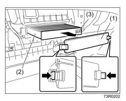
2) Remove the cover (1) and pull out the air conditioner filter (2).
