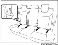
Your vehicle is equipped with the lower anchorages in the 2nd row seat outboard seating positions for securing a ISOFIX type of child restraints with the connecting bars. The lower anchorages are located where the rear of the seat cushion meets the bottom of the seatback.
