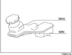
Check the brake fluid level by looking at the reservoir in the engine compartment. Check that the fluid level is between "MAX" and "MIN" lines
