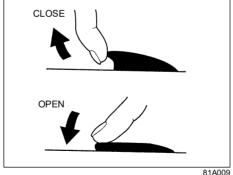
To open a window, push the top part of the switch. To close the window, lift up the top part of the switch.
