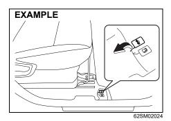
You can also unlatch the tailgate by pulling the release lever located on the outboard side of the driver's seat.
