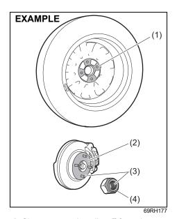
5) Clean any mud or dirt off from the surface of the wheel (1), hub (2), thread part (3) and surface of the wheel nuts (4) with a clean cloth. Clean the hub carefully; it may be hot from driving.
