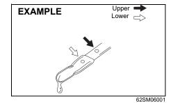
It is important to keep the engine oil at the correct level for proper lubrication of your vehicle's engine. Check the oil level with the vehicle on a level surface. The oil level indication may be inaccurate if the vehicle is on a slope. The oil level should be checked either before starting the engine or at least 5 minutes after stopping the engine.
