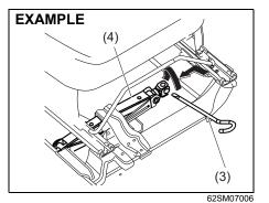
After temporarily holding the jack (4) until it contacts the storage bracket, turn the shaft approximately 60° to 90° by using jack handle (3) to securely hold the jack in place.
