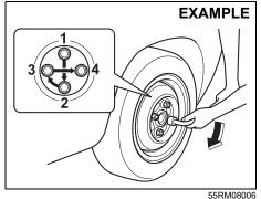
Tightening torque for wheel nut 100 Nm (10.1 kg-m, 73.7 lb-ft)
