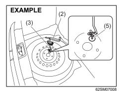
NOTE: If it is difficult to turn the bolt (5) by hand, use tools has shown in above illustration.
