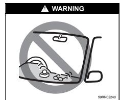
If you place any objects on the instrument panel, these objects may move and interfere with driver's view or safe driving. Also, the front passenger's front airbag may not work properly or these objects may be thrown out when the airbag inflates in an accident. Do not place any objects on the instrument panel.
