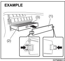
2) Remove the cover (1) and pull out the air conditioner filter (2).
