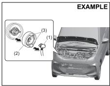
1) Open the engine hood while the engine is stopped. Disconnect the coupler (1). Remove the sealing rubber (2) by pulling the grip (3).
