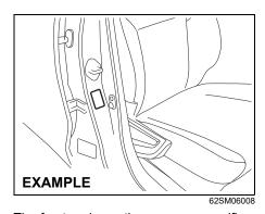
The front and rear tire pressure specifications are listed on the tire information label. Both front and rear tires should have the specified tire pressure.
