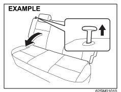
2) Pull the release knob(s) on the top of the seat(s) and fold the seatback forward.
