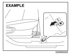
The fuel filler cap is located on the left rear side of the vehicle. The fuel filler door can be unlocked by pulling up the opener lever located on the outboard side of the driver's seat and locked by simply closing the door.
