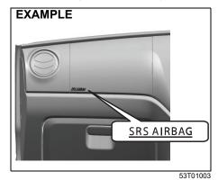
The driver's front airbag is located behind the center pad of the steering wheel and the front passenger's front airbag is located behind the passenger's side of the dashboard.
