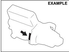
The engine serial number is stamped on the cylinder block as shown in the illustration.
