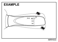
With the headlights on, push the lever forward to switch to the high beams (main beams) or pull the lever toward you to switch to the low beams. When the high beams (main beams) are on, a light on the instrument cluster will come on, to momentarily activate the high beams (main beams) as a passing signal, pull the lever slightly toward you and release it when you have completed the signal.
