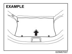
To remove the luggage compartment carpet (if equipped) easily, lift the carpet through the hole provided on the carpet and pull it out.
