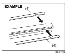
4) If the new blade is provided without the two metal retainers (4), move them from the old blade to the new one.
