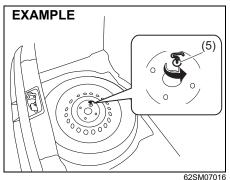
To remove the spare tire, turn its bolt (5) counterclockwise by hand.
