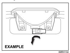
2) Remove the bulb holder as shown in the illustration.
