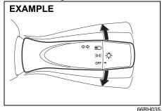
Move the lever all the way upward or downward to signal. When the turn is completed, the signal will cancel and the lever will return to its normal position.
