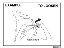
To lengthen, release the latch plate from the buckle, pull the latch plate (adjuster) in the direction of the arrow, at right angles to the belt. The latch plate should then be refitted into the buckle and the belt tightened as previously described.
