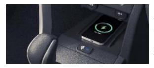
**Wireless Charging Dock** with LED indicator helps in seamless and comfortable charging of Qi certified phones. It also features **device left alert system.** The advanced system has a built-in safety feature that helps to safeguard the phones from overheating.
