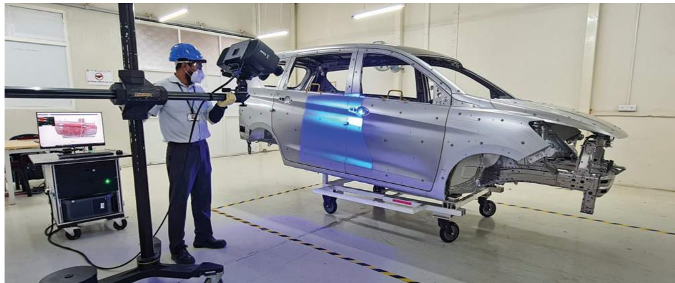
3D scanning room for product quality checks at Manesar facility
