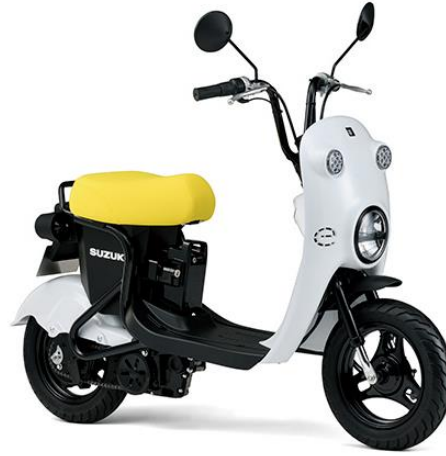
e-choinori, close distance mobility utilizing e-bike powertrain unit
