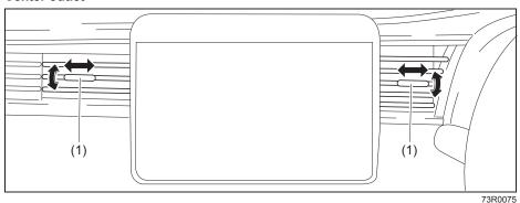
Move the knob (1) vertically or horizontally to adjust the direction of air flow as desired.
