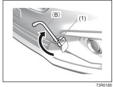
4) To tighten the towing eye (1), turn it clockwise by using a wheel wrench (B) until the towing eye (1) is securely installed.
