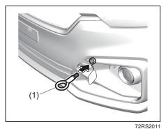
3) Install the towing eye (1) by hand.
