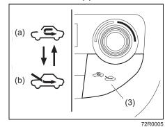
Push the air intake selector (3) to change between the recirculated air and fresh air
