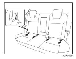
Your vehicle is equipped with the lower anchorages in the 2nd row seat outboard seating positions for securing a ISOFIX type of child restraints with the connecting
