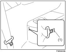
1) Insert the tongue plate of the buckle into the part (1)
