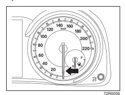
The speedometer indicates vehicle speed in km/h
