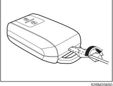
1) Insert a flat blade screwdriver covered with a soft cloth in the slot of the remote controller and pry it open.
