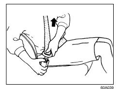
To unfasten the seat belt, push the button on the buckle and retract the belt slowly while attaching a hand to the belt or/and the latch plate.
