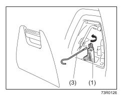
To remove the jack (1), turn its shaft counterclockwise by using jack handle (3) and pull the jack out of the storage bracket.
