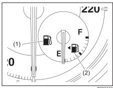
When the ignition switch is in "ON" position or the ignition mode is "ON", this gauge gives a rough indication of the amount of fuel in the fuel tank, "F" stands for full and "E" stands for empty.
