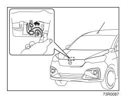
Push the under-hood release lever leftward with your finger, as shown in the illustration. While pushing the lever, lift up the engine hood.
