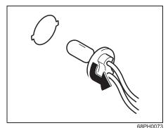
Open the engine hood while the engine is stopped. To remove the bulb holder of the front turn signal light or the front position light from the light housing, turn the holder counterclockwise and pull it out.
