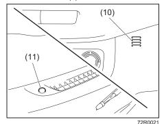
Be careful not to cover the interior temperature sensor (10) located between the steering wheel and the climate control panel, or the solar sensor (11) located at the top of the driver's side dashboard. These sensors are used by the automatic system to regulate temperature.
