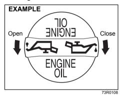
Remove the oil filler cap and pour oil slowly through the filler hole to bring the oil level to the upper limit on the dipstick. Be careful not to overfill the oil. Too much oil is almost as bad as too little oil. After refilling, start the engine and allow it to idle for about a minute. Stop the engine, wait about 5 minutes and check the oil level again. **Changing Engine Oil and Filter**
