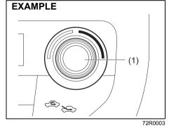
Turn the temperature selector (1) to adjust the temperature.
