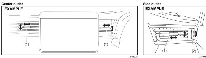
Move the knob (1) vertically or horizontally to adjust the direction of air flow as desired.
