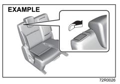
The walk-in type seat can be moved to provide easy entry to and exit from the 3rd row seats. You can move a walk-in seat by lifting up the release lever and pushing the seatback forward.
