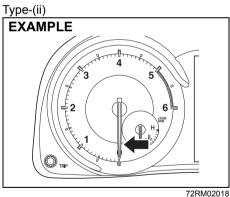
The tachometer indicates engine speed in revolutions per minute.
