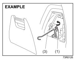
To remove the jack (1), turn its shaft counterclockwise by using jack handle (3) and pull the jack out of the storage bracket.
