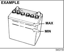
For maintenance-free battery (cap-less type), you need not add water. For traditional type battery, which has water filler caps, the level of the battery fluid must be kept between the "MAX" and the "MIN" level lines at all times. You should periodically check the battery, battery terminals, and battery hold-down bracket for corrosion. Remove corrosion using a stiff brush and ammonia mixed with water, or baking soda mixed with water. After removing corrosion, rinse with clean water.
