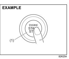
The "PUSH" indicator light in the instrument cluster will come on. Push the engine switch (1). When the engine is started, the starter motor will automatically stop.
