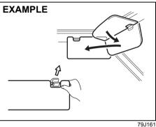
The sun visors can be pulled down to block glare coming through the windshield, or they can be unhooked and turned to the side to block glare coming through the side window.
