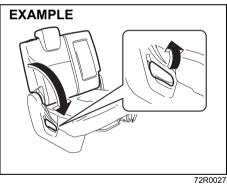
4) Pull up the lever on the outboard side of the seat, and fold the seatback forward.
