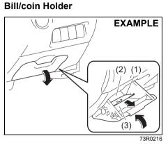
Pull the upper portion of the holder, downward to open the cover.
