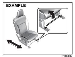
The adjustment lever for each front seat is located under the front of the seat. To adjust the seat position, pull up on the adjustment lever and slide the seat forward or rearward.
