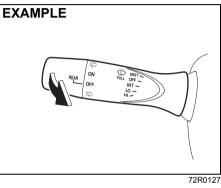
To spray windshield washer fluid, pull the lever toward you. The windshield wipers will automatically turn on at low speed if they are not already on and "INT" position is equipped.
