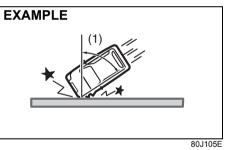
· Collision with a fixed wall or guardrail at left and right angles of greater than about 30 degrees (1) from the front of your vehicle
