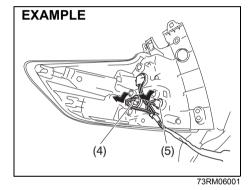
To remove the bulb holder of the rear turn signal light (4) or the reversing light (5) from the light housing, turn the holder counterclockwise and pull it out.
