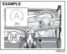
Regardless of whether the vehicle has stopped or not, depressing the clutch pedal will restart the engine and ENG A-STOP indicator light (green) (1) will go off.
