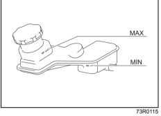
Check the clutch pedal for smooth operation and clutch fluid level from time to time. If clutch dragging is felt with the pedal fully depressed, have the clutch inspected by your Maruti Suzuki authorised workshop. If the clutch fluid level is near the "MIN" line, fill it up to the "MAX" line with Maruti Genuine Brake Fluid (MGBF) or DOT 3. We highly recommend to use "Maruti Genuine Brake Fluid" (MGBF).
