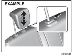
To raise the rear head restraint, pull upward on the restraint until it clicks. To lower the restraint, push down on the restraint while holding in the lock lever. If a head restraint must be removed (for cleaning, replacement, etc.), push in the lock lever and pull the head restraint all the way out.
