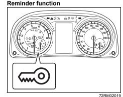
If the remote controller is not in the vehicle under the following conditions, the buzzer sounds intermittently for about 2 seconds and the immobilizer/keyless push start system warning light on the instrument cluster blinks:
