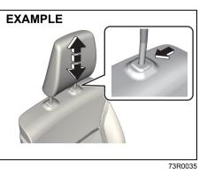
To raise the front head restraint, pull upward on the restraint until it clicks. To lower the restraint, push down on the restraint while holding in the lock lever. If a head restraint must be removed (for cleaning, replacement, etc.), push in the lock lever and pull the head restraint all the way out.
