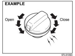
To remove the fuel filler cap:
