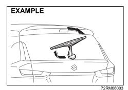
2) Remove the wiper frame from the wiper arm as shown.
