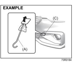
2) Remove the cover (C) by using a jack handle (A) covered with a soft cloth as shown in the illustration.
