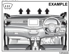
Temperature-controlled air comes out of the windshield defroster outlets, the side defroster outlets and the side outlets.
