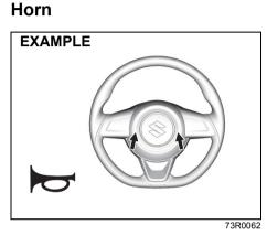
Press the horn button of the steering wheel to sound the horn. The horn will sound with the ignition switch in any position or any ignition mode.
