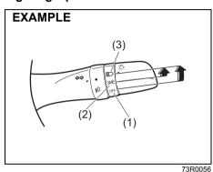
To turn the lights on or off, twist the knob on the end of the lever. There are three positions:
