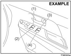
The driver's door has a switch (1) to operate the driver's window, and a switch (2) to operate the front passenger's window and there are switches (3) and (4) to operate the rear right and left passenger windows, respectively.
