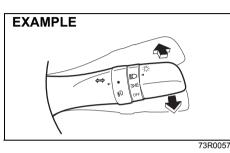
With the headlights on, push the lever forward to switch to the high beams (main beams) or pull the lever toward you to switch to the low beams. When the high beams (main beams) are on, a light on the instrument cluster will come on. To momentarily activate the high beams (main beams) as a passing signal, pull the lever slightly toward you and release it when you have completed the signal.
