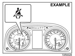
When the driver and/or front passenger do(does) not fasten their seat belts, the seat belt reminder lights will come on or blink and a buzzer will sound to remind the driver and/or passenger to fasten their seat belts. For more details, refer to the explanation below.
