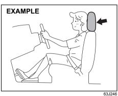
Head restraints are designed to help reduce the risk of neck injuries in the case of an accident. Adjust the head restraint to the position which places the center of the head restraint closest to the top of your ears. If this is not possible for very tall passengers, adjust the head restraint as high as possible.
