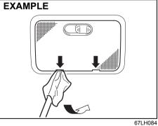
Remove the lens by using a flat-bladed screwdriver covered with a soft cloth as shown. To install it, simply push it back in.
