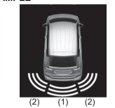
· Warnings when obstacles such as wall are detected by corner sensors
