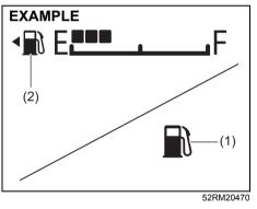
When the ignition switch is in "ON" position, this gauge gives a rough indication of the amount of fuel in the fuel tank. "F" stands for full and "E" stands for empty.
