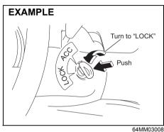
• **Manual Transmission vehicles** You must push in the key to turn it to LOCK position. It locks the ignition, and prevents normal use of the steering wheel after the key is removed.
