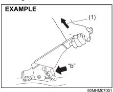
Ratchet tooth specification "b": 4th – 9th Lever pull force (1): 200 N (20 kg, 45 lbs)
