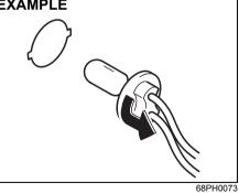
1) Open the engine hood while the engine is stopped. To remove the bulb holder of the front turn signal light or the front position light from the light housing, turn the holder counterclockwise and pull it out.
