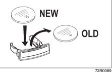
2) Remove the old battery and place the new battery (CR2025) into the battery slot cover with the + mark facing upwards.
