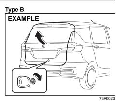
To open the tailgate, insert the key and turn it clockwise to unlatch and lift the tailgate.
