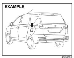
The fuel filler cap is located on the left rear side of the vehicle. The fuel filler door can be unlocked by pulling up the opener lever located on the outboard lower side of the driver's seat and locked by simply closing the door.
