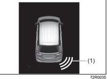
(1) Symbol representing an obstacle detected by parking sensor\*
