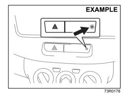
This light will blink with the ignition switch in LOCK or ACC position, or the ignition mode "LOCK" (OFF) or "ACC". The blinking light is intended to deter theft by leading others to believe that the vehicle is equipped with a security system.
