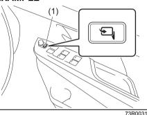
You can fold the mirrors when you park the vehicle in a narrow space. When the ignition switch is in the ACC or ON position, or the ignition mode is "ACC" or "ON", push the folding switch (1) to fold and unfold the mirrors.
