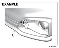
The towing eye (1) is provided on the front of the vehicle for use in emergency situations and sea shipping purpose only.
