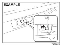
2) Open the cover (2) in the lock mechanism of the tailgate.
