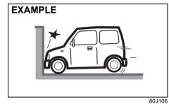
Frontal collision with a fixed wall that does not move or deform at less than about 25 km/h
