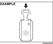
To stow the key into the remote controller, push the key in the remote controller until you hear a click.
