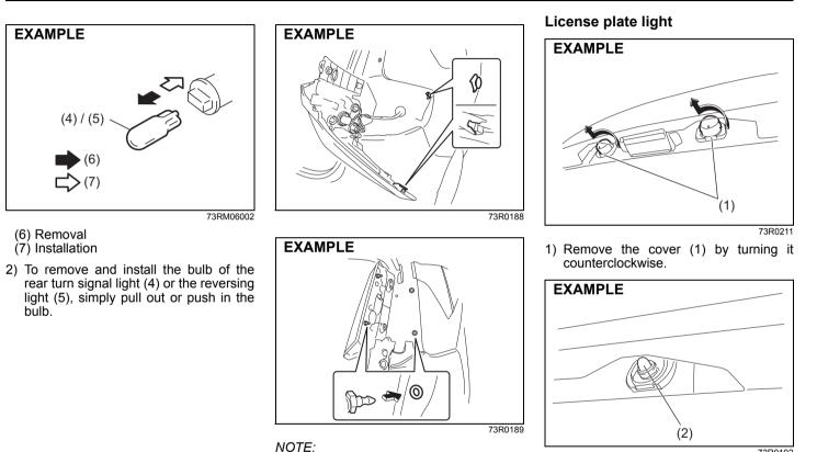
When reinstalling the light housing, check that the clips are properly attached.
