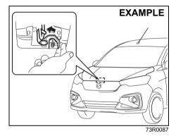
Push the under-hood release lever leftward with your finger, as shown in the illustration. While pushing the lever, lift up the engine hood.
