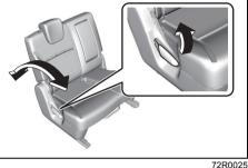
To adjust the seatback angle of 2nd row seats, pull up the lever on the outboard side of the seat, move the seatback to the desired position, and release the lever to lock the seatback in place.
