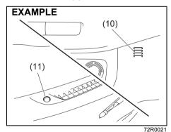
Be careful not to cover the interior temperature sensor (10) located between the steering wheel and the climate control panel, or the solar sensor (11) located at the top of the driver's side dashboard. These sensors are used by the automatic system to regulate temperature. Even if the engine is turned OFF, the tem-
