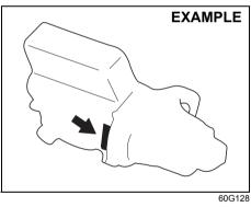
The engine serial number is stamped on the cylinder block as shown in the illustration.
