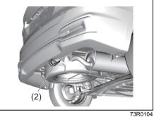
The frame hook (2) is provided on the rear of the vehicle for use in emergency situations and sea shipping purposes only.
