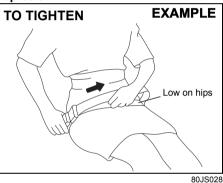
Sit up straight and well back in the seat. To fasten the belt, pull the latch plate attached to the seat belt across your hips and press it straight into the buckle until you hear a "click". To reduce the risk of sliding under the belt during a collision, position the belt across your lap as low on your hips as possible and adjust it to a snug fit. To tighten the belt, pull the free end of the belt across alongside the lap strap.
