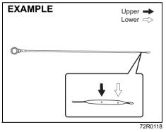
It is important to keep the engine oil at the correct level for proper lubrication of your vehicle's engine. Check the oil level with the vehicle on a level surface. The oil level indication may be inaccurate if the vehicle is on a slope. The oil level should be checked either before starting the engine or at least 5 minutes after stopping the engine.
