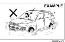
Avoid driving in a flooded area or a deep puddle. If driving in a flooded area is unavoidable, go slowly in the lowest gear. In case that you have driven in a flooded area, stop the vehicle in a safe and non flooded place while checking the brake effectiveness. Then, ask a Maruti Suzuki authorised workshop to check the following inspection items.
