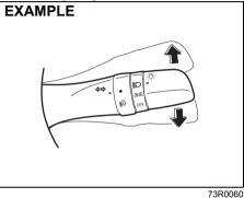
Move the lever partially upward or downward to turn right or left and hold the lever in the moved position.
