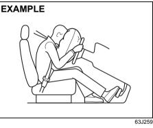
Front airbag is designed to inflate in severe frontal collisions when the ignition switch is in "ON" position or the ignition mode is "ON".
