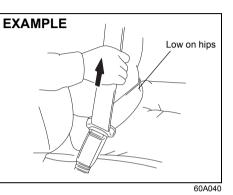
To reduce the risk of sliding under the belt during a collision, position the lap portion of the belt across your lap as low on your hips as possible and adjust it to a snug fit by pulling the shoulder portion of the belt upward through the latch plate. The length of the diagonal shoulder strap adjusts itself to allow freedom of movement.
