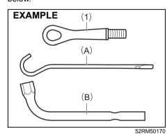
Pick up the towing eye (1), jack handle (A) and wheel wrench (B) in the luggage compartment.
