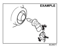
Open the fender cover. Disconnect the coupler with pushing the lock release. Turn the bulb holder counterclockwise and remove it.
