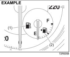
When the ignition switch is in "ON" position or the ignition mode is "ON", this gauge gives a rough indication of the amount of fuel in the fuel tank. "F" stands for full and "E" stands for empty.
