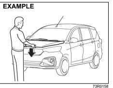
2) Lower the hood to about 20 cm above the hood latch, and then let it drop down. Make sure the hood is securely latched after closing.
