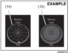
The meter indication is different depending on whether the vehicle is stopped or running.
