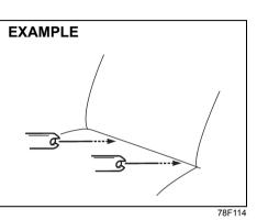
Place the child restraint in the 2nd row seat, inserting the connecting bars to the anchorages between the seat cushion and the seatback.
