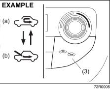
Push the air intake selector (3) to change between the recirculated air and fresh air mode.
