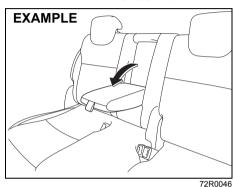
The rear armrest is stowed in the center of the seatback. Tilt it down forward to use.
