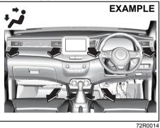
When the temperature selector (1) is in the fully cold position or fully hot position, however, the air from the floor outlets and the air from the center, side and cup holder outlets will be the same temperature. HEAT (e)
