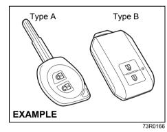
Your vehicle is equipped with either a keyless entry system transmitter (Type A) or a keyless push start system remote controller (Type B). The transmitter has only a keyless entry function. The remote controller has a keyless entry function and a keyless push start system. The transmitter has only a keyless entry function. For details, refer to the following explanations.
