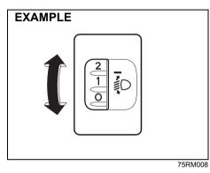
Level the headlight beam according to the load condition of your vehicle by turning this switch. The chart shows the appropri-ate switch position for different vehicleload conditions.
