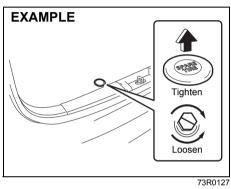
Remove the cap and use a wheel wrench to loosen the hook bolt of the spare tire holder. Then, rotate using the end of the jack handle.
