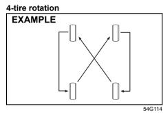
To avoid uneven wear of your tires and to prolong their life, rotate the tires as illustrated. Tires should be rotated every 10000 km. After rotation, adjust front and rear tire pressures to the specification listed in your vehicle's Tire Information Label.
