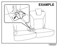
2) Stow the seat belt buckles of the right and left seating position into the pocket of the seat cushion as shown in the illustration.
