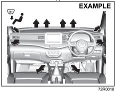
Temperature-controlled air comes out of the floor outlets, the windshield defroster outlets, the side defroster outlets and the side outlets.
