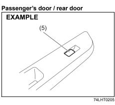
The passenger's door has a switch (5) to operate the passenger's window.
