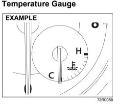
When the ignition switch is in "ON" position or the ignition mode is "ON", this gauge indicates the engine coolant temperature. Under normal driving conditions, the indicator should stay within the normal, acceptable temperature range between "H" and "C". If the indicator approaches "H", overheating is indicated. Follow the instructions for engine overheating in "EMERGENCY SERVICE" section.
