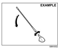
The radio antenna on the roof is removable. To remove the antenna, turn it counterclockwise. To reinstall the antenna, turn it clockwise firmly by hand.
