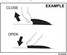
To open a window, push the top part of the switch. To close the window, lift up the top part of the switch.
