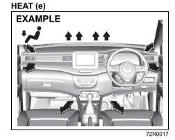
Temperature-controlled air comes out of the floor outlets and the side outlets, also comes out of the windshield defroster outlets and the side defroster outlets slightly. HEAT & DEFROST (f)
