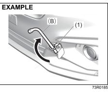
To tighten the towing eye (1), turn it clockwise by using a wheel wrench (B) until the towing eye (1) is securely installed.
