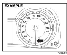
The speedometer indicates vehicle speed in km/h.
