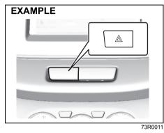
Push the hazard warning switch to activate the hazard warning lights. All turn signal lights and both turn signal indicators will flash simultaneously. To turn off the lights, push the switch again.
