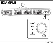
To turn on the overhead rear air conditioning system, set the blower speed selector of the heating and air conditioning system to a position other than off and push in "A/ C" switch. Refer to "Air conditioning switch" in this section. And set the rear blower speed selector (2) to a position other than off.
