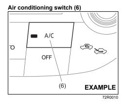
The air conditioning switch (6) is used to turn on and off the air conditioning system only when the blower is on. To turn on the air conditioning system, push in the switch and "A/C" will appear in the display. To turn off the air conditioning system, push in the switch again and "A/C" will go off. System Operating Instructions
