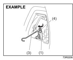
After temporarily holding the jack (1) until it contacts the storage bracket, turn the shaft (4) approximately 90° to 180° by using jack handle (3) to securely hold the jack in place.
