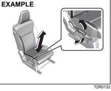
If the driver's seat is equipped with a seat height adjuster lever on the outboard side of the seat, raise or lower the seat by pulling up or down the adjuster lever.
