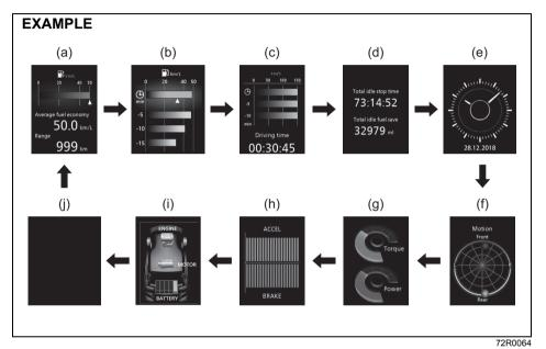
To switch the display indication, push the indicator selector knob (3) quickly.
