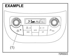
When the rear window is misted, push this switch (1) to clear the window.
