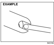
Push the child restraint toward the anchorages so that the connecting bar tips are partially hooked to the anchorages. Use your hands to confirm the position.
