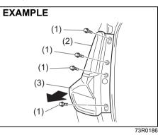
With the tailgate opened, remove the bolts (1) and tail light (2), and then pull the rear combination light (3) firmly to the rearward.
