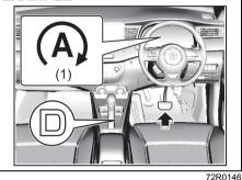
While depressing the brake pedal, place the gearshift lever in "D" or "N" position.
