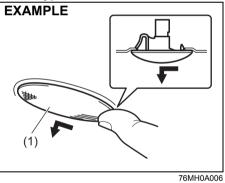
1) Remove the side turn signal light assembly (1) by sliding light housing to left with your finger.
