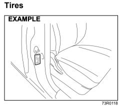
The front and rear tire pressure specifications for your vehicle are listed in the tire information label. Both front and rear tires should have the specified tire pressure.
