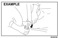
To fasten the seat belt, sit up straight and well back in the seat, pull the latch plate attached to the seat belt across your body and press it straight into the buckle until you hear a "click".
