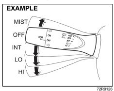
To turn the windshield wipers on, move the lever down to one of the three operating positions. In "INT" position, the wipers operate intermittently. "INT" position is very convenient for driving in mist or light rain. In "LO" position, the wipers operate at a steady low speed. In "HI" position, the wipers operate at a steady high speed. To turn off the wipers, move the lever back to "OFF" position.
