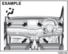
Temperature-controlled air comes out of the floor outlets and cooler air comes out of the center, side and cup holder outlets. When the temperature selector (1) is in the fully cold position or fully hot position, however, the air from the floor outlets and the air from the center, side and cup holder outlets. will be the same temperature.
