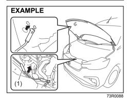
3) While holding the hood, pull the prop rod out from the holding clip by protector (1), and then insert the end of the
