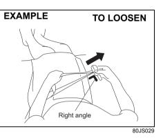
To lengthen, release the latch plate from the buckle, pull the latch plate (adjuster) in the direction of the arrow. The latch plate should then be refitted into the buckle and the belt tightened as previously described. To unfasten the belt, press the release button and the buckle latch.
