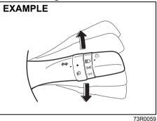
Move the lever all the way upward or downward to signal. When the turn is completed, the signal will cancel and the lever will return to its normal position.
