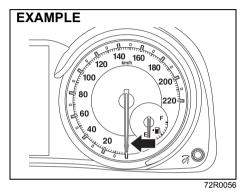
The speedometer indicates vehicle speed in km/h.
