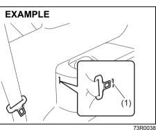
1) Insert the tongue plate of the buckle into the part (1).
