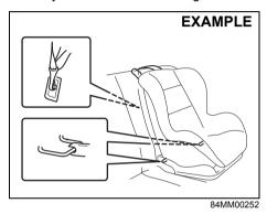
Your vehicle is equipped with the top tether anchorages. Use the top tether strap of the child restraint according to the instructions provided by the child restraint system manufacturer.
