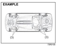
The frame holes (3) are provided only for transporting by a car carrier trailer.
