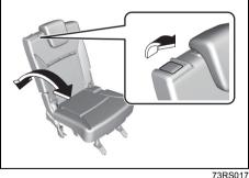
To adjust the seatback angle of 3rd row seats, put one hand on the backrest and fully lift up the release lever in the upper side of the backrest.
