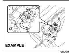
(1) Fuel filter(2) Fuel inlet hose(3) Fuel outlet hose
