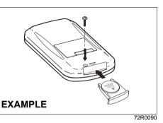
Press the battery slot cover to the direction indicated by the arrow completely and then fully tighten the screw.
