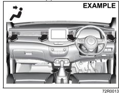
Temperature-controlled air comes out of the center, side and cup holder outlets.
