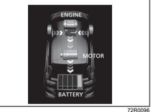
While decelerating your vehicle, the ISG generates electricity without engine power. This reduces engine loads and improves fuel consumption.
