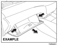
To approach the air conditioner filter, remove the glove box by pressing both sides of the glove box inward and pull-
