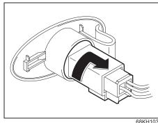
To remove a bulb holder from a light housing, turn the holder clockwise and pull it out. Then remove the bulb. Install a new bulb in the reverse order.
