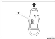
To remove the key from the remote control-Ier, push the button (A) in the direction of the arrow and pull the key out from the remote controller.
