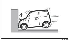
. In frontal collisions with a fixed wall that does not move or deform in more than about 25 km/h (15 mph)
