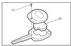
If the transmitter battery gets discharged, replace the battery with a new one.
