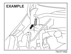
The chassis and/or engine serial numbers are used to register the vehicle. They are also used to assist your dealer when ordering or referring to special service information. Whenever you have occasion to consult your MARUTI SUZUKI dealer, remember to identify your vehicle with this number. Should you find the number difficult to read, you will also find it on the identification plate.
