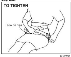
fasten the belt, pull the latch plate attached to the seat belt across your hips and press it straight into the buckle until you hear a "click". To reduce the risk of sliding under the belt during a collision, position the belt across your lap as low on your hips as possible and adjust it to a snug fit. To tighten the belt, pull the free end of the
