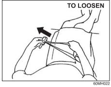
To lengthen, release the latch plate from the buckle, pull the latch plate (adjuster) in the direction of the arrow. The latch plate should then be refitted into the buckle and the belt tightened as previously described.
