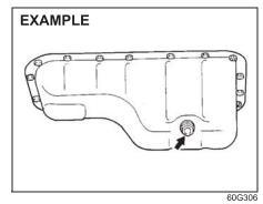
Tightening torque for drain plug Petrol engine: 35 Nm (3.5 kg-m, 25.3 lb-ft) Diesel engine:
