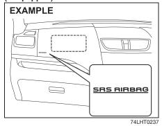
The driver's front air bag is located behind the center pad of the steering wheel and the front passenger's front air bag (if
