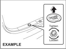
1) Remove the cap and loosen the spare tire holder hook bolt with the lug wrench.
