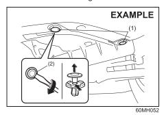
Insert a flat blade screwdriver into the hole (2) and remove the clips (1) by twist the driver as shown in the illustration.
