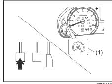
Depress the clutch pedal while the gearshift lever is in the "N" (Neutral) position. "ENG A-STOP" indicator light (green) (1) in the instrument cluster will be turned off and the engine will restart automatically.
