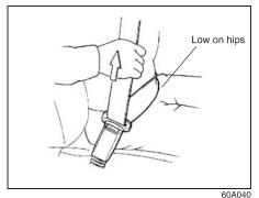
To reduce the risk of sliding under the belt during a collision, position the lap portion
