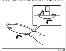
Remove the light housing by sliding to left with your finger.
