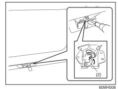
2) Push open the tailgate from inside by pushing up on the emergency lever (2) using a flat blade screwdriver or the jack handle. The tailgate will be latched again by closing the tailgate simply.
