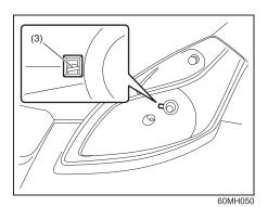
NOTE: You can see the position of retaining spring (3) from the hole of headlight.
