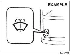
Check that there is washer fluid in the tank. Refill it if necessary. Use a good quality windshield washer fluid, diluted with water as necessary.
