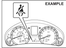
When the driver does not buckle his or her seat belt, the driver's seat belt reminder light in the instrument cluster will come on or blink and a buzzer will sound as a reminder to the driver to buckle his or her seat belt. For more details, refer to the explanation below.
