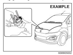
2) Push the under-hood release lever sideways with your finger, as shown in the illustration. While pushing the lever, lift up the engine hood.
