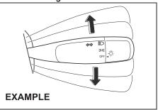
Move the lever all the way upward or downward to signal. When the turn is completed, the signal will cancel and the lever will return to its normal position.
