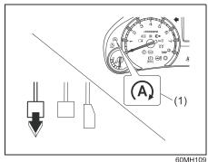
3) Release the clutch pedal. The "ENG A-STOP" indicator light (green) (1) in the instrument cluster will illuminate and the engine will stop automatically.
