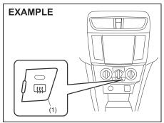
When the rear window is misted, push this switch (1) to clear the window.
