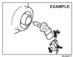
3) Open the fender cover. Disconnect the coupler with pushing the lock release. Turn the bulb holder counterclockwise and remove it.
