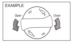
Remove the oil filler cap and pour oil slowly through the filler hole to bring the oil level to the upper limit on the dipstick. Be careful not to overfill. Too much oil is almost as bad as too little oil. After refilling, start the engine and allow it to idle for about a minute. Stop the engine, wait about 5 minutes and check the oil level again.
