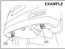
The frame hook (3) is provided on the rear of the vehicle for use in emergency situations and trailer/train/sea shipping purposes only.
