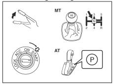
1) Make sure the parking brake is set fully. tral) and depress the clutch pedal all
