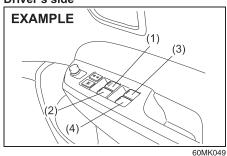
ate the driver's window, and a switch (2) to operate the front passenger's window or there are switches (3), (4), to operate the rear right and left passenger windows, respectively.
