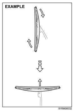
3) Install wiper frame to arm in the reverse order of removal.
