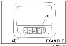
The dashboard has a switch(1) to operate the driver's window and a switch(2) to operate the front passenger's window. To open a window, push the bottom part (b) of the switch. To close the window, push the part (a) of the switch.
