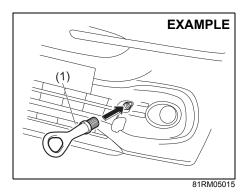
3) Install the towing hook (1) by hand.
