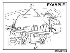
1) Unhook air cleaner case clamps (1). Open air cleaner case (2) and then remove air cleaner filter.
