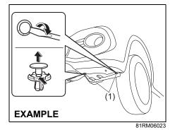
Remove the clip (1) by prying it off with a flat-bladed screwdriver as shown in the illustration.
