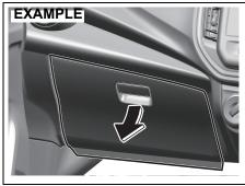
To open the glove box, pull the latch lever. To close it, push the lid until it latches securely.
