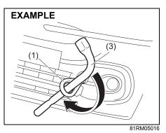
To tighten the towing hook (1), turn it clockwise by using a wheel brace (3) until the towing hook (1) is securely installed.
