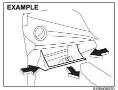
1) To approach the air conditioner filter, remove the glove box. Press both sides of the glove box in arrow direction to remove it.
