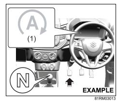
Regardless of whether the vehicle has stopped or not, depressing the clutch pedal will restart the engine and ENG A-STOP indicator light (green) (1) will go off. While the engine is stopped automatically, depressing the clutch pedal will restart the engine consuming fuel. Therefore, for fuel economy, it is recommended to depress the clutch pedal just before the vehicle start.
