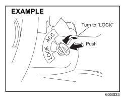
You must push in the key to turn it to "LOCK" position. It locks the ignition, and prevents normal use of the steering wheel after the key is removed.
