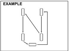
prolong their life, rotate the tires as illustrated. Tires should be rotated as mentioned in periodic maintenance schedule. After rotation, adjust front and rear tire pressures to the specification listed on your vehicle's tire information label.
