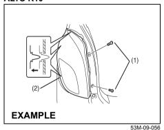
Remove the screw (1). Remove the combination light (2) by pulling it outside.
