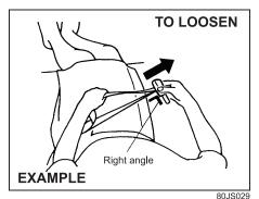
To lengthen, release the latch plate from the buckle, pull the latch plate (adjuster) in the direction of the arrow, at right angles to the belt. The latch plate should then be refitted into the buckle and the belt tightened as previously described.
