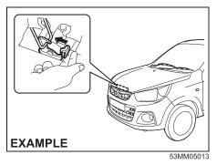
2) Push the under-hood release lever sideways with your finger, as shown in the illustration. While pushing the lever, lift up the engine hood.
