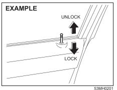
To lock a door from inside the vehicle, push the lock knob down. Pull the lock knob up to unlock the door.
