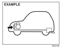
The purpose of the catalytic converter is to minimize the amount of harmful pollutants in your vehicle's exhaust. Use of leaded fuel in vehicles equipped with catalytic converters is prohibited, because lead deactivates the pollutant-reducing components of the catalyst system.
