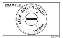
The ignition switch has the following four positions:
