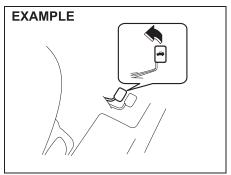
You can also unlatch the tailgate by pulling the release lever (if equipped) located on the outboard side of the driver's seat.
