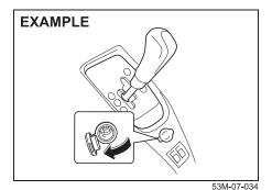
The accessory socket will work when the ignition switch is in the "ACC" or "ON" position. This socket can be used to provide 12volt/120 watt power for electrical accessories. Check that the cap remains on the socket when socket is not in use.
