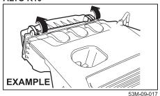
Unclamp/Unscrew the side clamps/screws, and remove the element from the air cleaner case. If it appears to be dirty, replace it with a new one.
