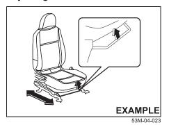
The adjustment lever for each front seat is located under the front of the seat. To adjust the seat position, pull up on the adjustment lever and slide the seat forward or rearward.
