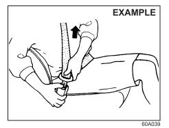
To unfasten the seat belt, push the red "PRESS" button on the buckle and retract the belt slowly while attaching a hand to the
