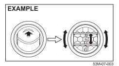
When "Open", air comes out regardless of the air flow selector position.
