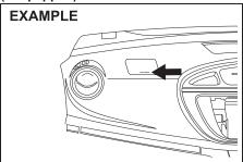
The driver's front air bag is located behind the center pad of the steering wheel and the front passenger's front air bag is located behind the passenger's side of the dashboard.
