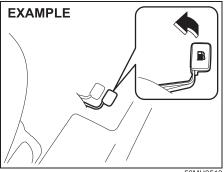
The fuel filler cap is located on the left rear side of the vehicle. The fuel filler door can be unlocked by pulling up the opener lever located on the outboard side of the driver's seat and locked by simply closing the door.
