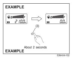
To reset the trip meter to zero, hold in the "MODE" knob (3) for about 2 seconds.
