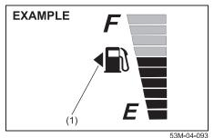
When the ignition switch is in the "ON" position, this gauge gives an approximate indication of the amount of fuel in the fuel tank. "F" stands for full and "E" stands for empty.
