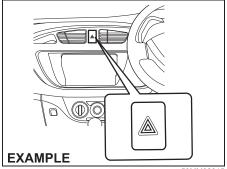
Push in the hazard warning switch to activate the hazard warning lights. All turn signal lights and both turn signal indicators will flash simultaneously. To turn off the lights, push the switch again.
