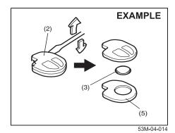
5) Close the transmitter and install it into
