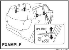
You can also lock or unlock doors by pushing down or pulling up the driver's door lock knob (1).
