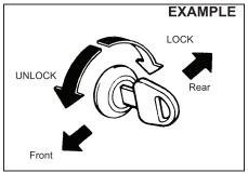
You can lock and unlock all doors simultaneously by using the key in the driver's door lock.
