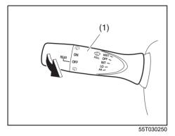
If you pull the lever (1) toward you, the windshield washer fluid will be sprayed and the windshield wipers will automatically operate a few times.
