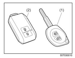
Your vehicle is equipped with either a keyless entry system transmitter (1) or a keyless push start system remote controller (2). The transmitter has only a keyless entry system. The remote controller has a keyless entry system and a keyless push start system. For details, refer to the following explanations.
