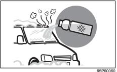
Melt ice by pouring lukewarm water. After melting it, wipe off water to prevent refreezing. If you operate the wiper blades forcedly when ice stays freezing, the wiper rubbers may be damaged and the wiper blades may be broken.
