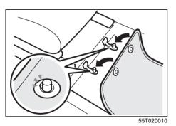
To prevent the driver's side floor mat from sliding forward and possibly interfering with the operation of the pedals, MARUTI SUZUKI genuine floor mats are recommended. Whenever you put the driver's side floor mat back in the vehicle after it has been removed, hook the floor mat grommets to the fasteners and position the floor mat properly in the footwell.
