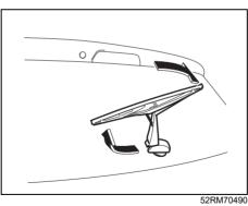
2) Remove the wiper frame from the wiper arm after rotating the wiper frame clockwise.
