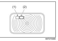
When you open the tailgate with the luggage compartment light switch in the "ON" position (1), the light comes on for about 15 minutes.
