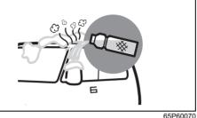
Melt ice by pouring lukewarm water. After melting it, wipe off water to prevent refreezing. If you operate the outside rearview mirrors forcedly when ice stays freezing, the outside rearview mirrors may be broken.
