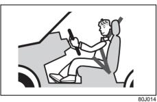
There is a possibility of major impact from the front airbags when the airbags activate and deploy instantaneously, the driver and the passenger should sit deeply into their seats and touch their backs lightly to the seatback. In addition, the seat should be positioned so that it is not too far forward.
