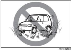
Do not drive in the field covered with grown grass If you drive in the field covered with grass, it may cause accident or fire or vehicle damage by getting caught in grown grass.
