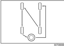
To avoid uneven wear of your tyres and to prolong their life, rotate the tyres as illustrated. Tyres should be rotated every 10000 km. After rotation, adjust front and rear type pressures to the specification listed on your vehicle's Tyre Information Label
