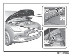
3) While holding the hood, pull the prop rod (3) out from the holding clip (4), and then insert the end of the rod into the designated hole (5).
