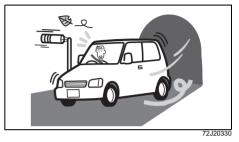
At a tunnel exit, on a bridge, or when a large truck passes you, your vehicle might be blown slightly sideways by side wind. Do not panic. Firmly grasp the steering wheel, gradually reduce speed, and regain your intended course.
