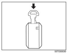
To stow the key into the remote controller, push the key in the remote controller until vou hear a click.
