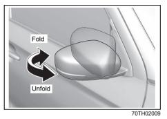
Position of switch Unfold Fold You can fold the mirrors when you park the vehicle in a narrow space. Push the folding switch to fold and unfold the mirrors. Make sure the mirrors are completely unfolded before you start driving.
