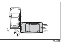
• Impact from the side to the vehicle body other than the passenger compartment
