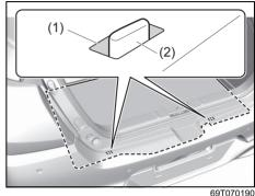
There is a tool box under the luggage compartment carpet. When installing the luggage compartment carpet, hook the carpet by using the holes (1) in the carpet, onto the hooks (2) at the base of the luggage compartment.
