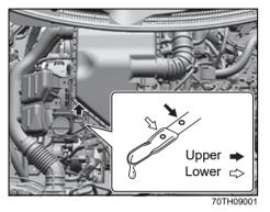
It is important to keep the engine oil at the correct level for proper lubrication of your vehicle's engine. Check the oil level with the vehicle on a level surface. The oil level indication may be inaccurate if the vehicle is on a slope. The oil level should be
