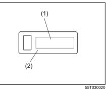
The key identification number (1) is stamped on a metal tag (2) provided with the keys. Keep the tag in a safe place. If you lose your keys, you will need this number to have new keys made. Write the number below for your future reference.
