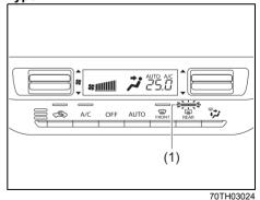
While the engine is running or the engine automatically stops by the ENG A-STOP system, you can use the heated rear window switch as the defogger for the rear window glass.
