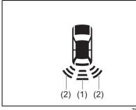
Upon detecting an obstacle, the parking sensor causes an interior buzzer to sound and a symbol representing the obstacle appears on the information display in the instrument cluster.
