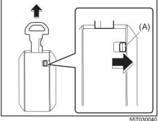
To remove the key from the remote controller, slide the lock knob (A) in arrow direction and pull the key out from the remote controller.
