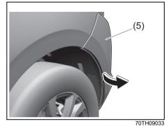
3) Open the end of the front bumper (5) in arrow direction.
