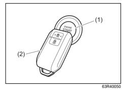
Manual transmission – Without depressing the clutch pedal, push the engine switch (1).
