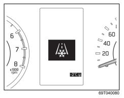
If the outside temperature nears freezing condition, the message shown in the above illustration will appear on the display.
