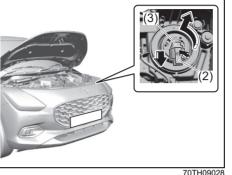
Disconnect the coupler (2) by pushing the lock release. Turn the bulb (3) counterclockwise and remove it.
