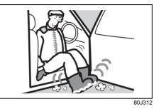
Remove snow attaching to shoes before getting in your vehicle. If you do not remove it, you may slip when operating the pedals and the window glasses may mist easily because of high humidity inside the vehicle.
