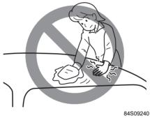
• When washing or waxing the vehicle, do not lean on the vehicle body or do not push it hard. This might cause it to deform. (Continued)
