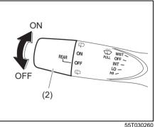
You can operate the rear window wiper by twisting the lever (2) as shown in the illustration
