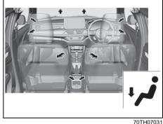
Temperature-controlled air comes out of the floor outlets and the side outlets, a small amount of air comes out of the windshield defroster outlets and also comes slightly out of the side and rear (if equipped) defroster outlets.
