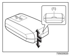
1) Pull the key out from the remote controller.  Separate the remote controller up and down while applying force to the slot (1) on the side of the remote controller.
