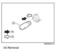
(5) Install3) To remove and install the bulb of the side turn signal light (3) simply pull out
