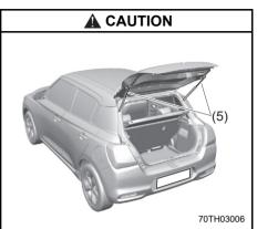
To avoid damage and malfunction of the dumper stay, observe the following precautions. Otherwise, the damper stay (5) which upholds the tailgate may not operate smoothly and the tailgate may not be kept up when opening it.
