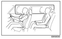
Side airbags and side curtain airbags are designed to inflate in severe side impact collisions when the ignition switch is in "ON" position or the ignition mode is ON.
