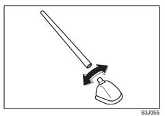
The radio antenna on the roof is removable. To remove the antenna, turn it counterclockwise. To reinstall the antenna, turn it clockwise firmly by hand. NOTICE
