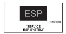
If the message shown in the above illustration appears on the information display, there may be a problem with the ESP<sup>®</sup> system. Have your vehicle inspected by a MARUTI SUZUKI authorized workshop (if equipped with instrument cluster type B).
