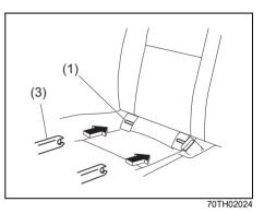
Place the child restraint in the rear seat, inserting the connecting bars (3) to the lower anchorages (1) between the seat cushion and the seatback.
