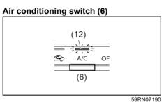
The air conditioning switch (6) is used to turn on and off the air conditioning system only when the blower is on. To turn on the air conditioning system, push in the switch and "A/C" will appear in the display. To turn off the air conditioning system, push in the switch again and "A/C" will go off.
