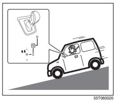
For Auto Gear Shift vehicle, shift the gearshift lever into "M" (manual mode) first. Then, pull "–" side of the shift paddle to shift down to an appropriate gear position.
