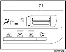
Push upper part or lower part of the temperature selector (1) to adjust the temperature.
